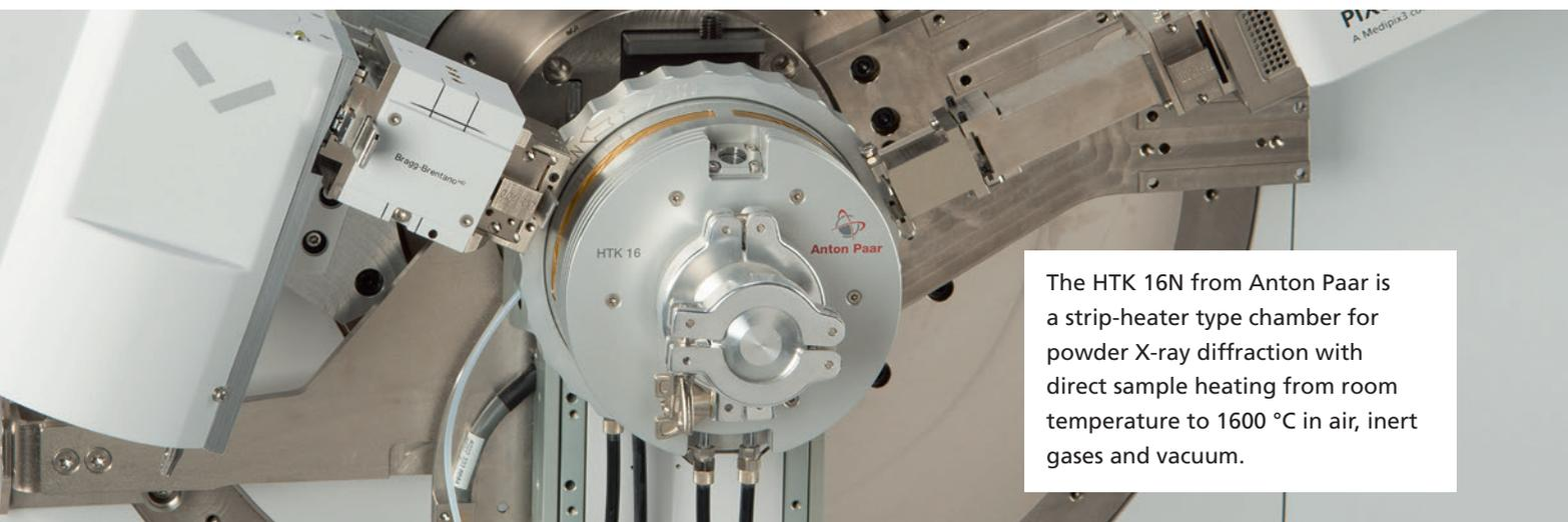
The HTK 16N from Anton Paar is a strip-heater type chamber for powder X-ray diffraction with direct sample heating from room temperature to 1600 °C in air, inert gases and vacuum.
